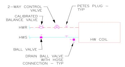
It is allowed to use a combination valve assembly such as the Flow Design Inc. model UA or UB with included NPT union connections and optional pressure/temperature ports, and manual air vent on the return water side. Model UA or UB with included NPT union connections and optional pressure/temperature ports, and hose end drain on the supply water side. Approval by Owner is required prior to installation.
